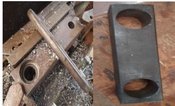
Fig.4(f) Milling Operation On Self Made Bearing Casing
