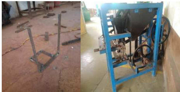
Fig.4.Fabricated model of the mango cutting machine
