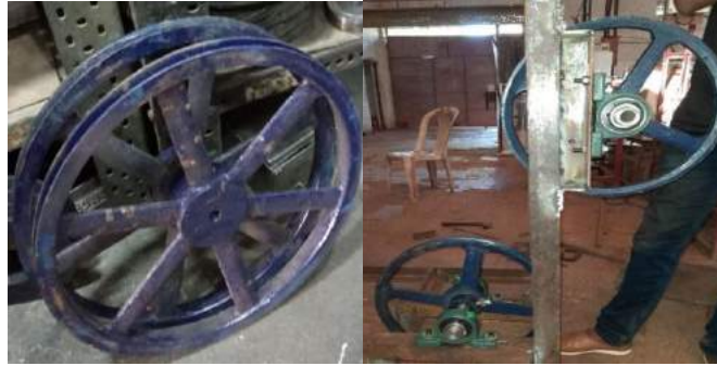
Fig.4(m) Standard Pulleys Fig.4(n) Pulleys Mounted On Frame
