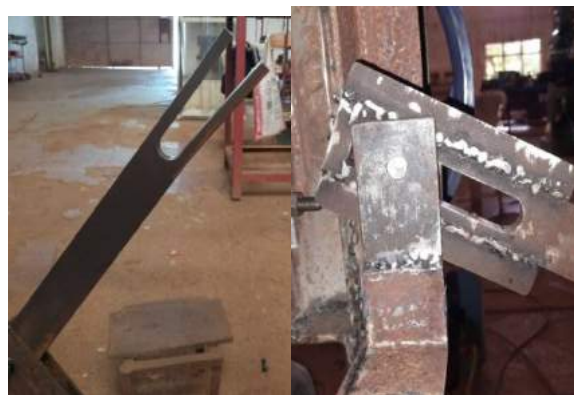
Fig.4 (k) Bending During Testing Fig.4 (l) Bending Overcome
