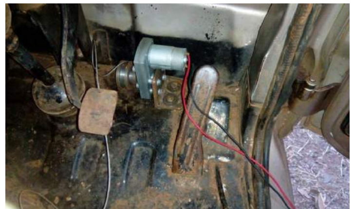
Figure 3: Position of Electric Motor for application of brake
