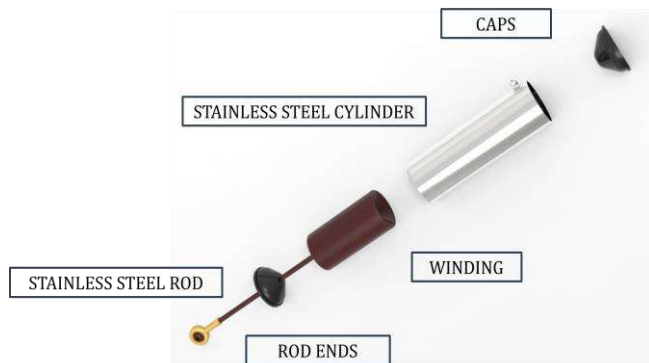
Fig.12: Electromagnetic Gear Shifter exploded view
