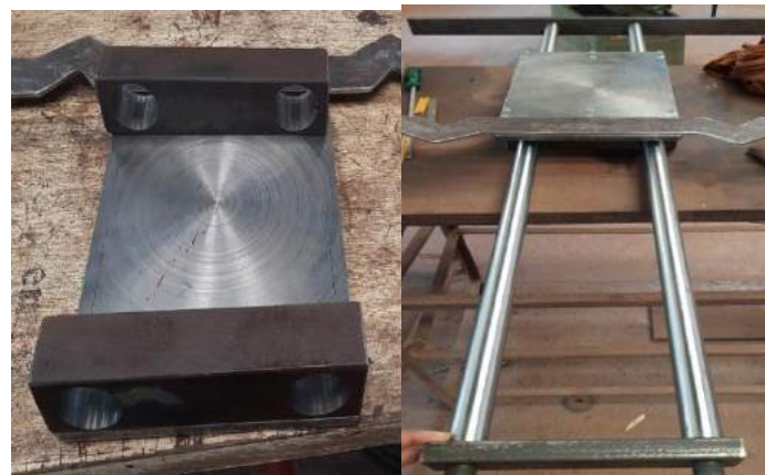
Fig.4 (g) Mounting All The Necessary Part On Moving Plateand Guide Bar
